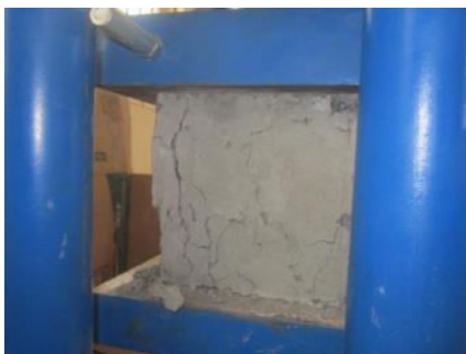
Figure.2 Test setup for compressive strength
